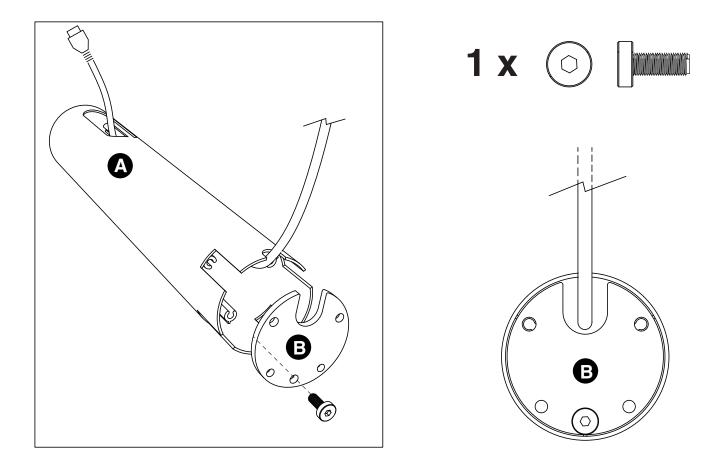
3. Join the 2 legs (C and D) and screw them to the tube through the steel disc (B), using the 4 long screws.
