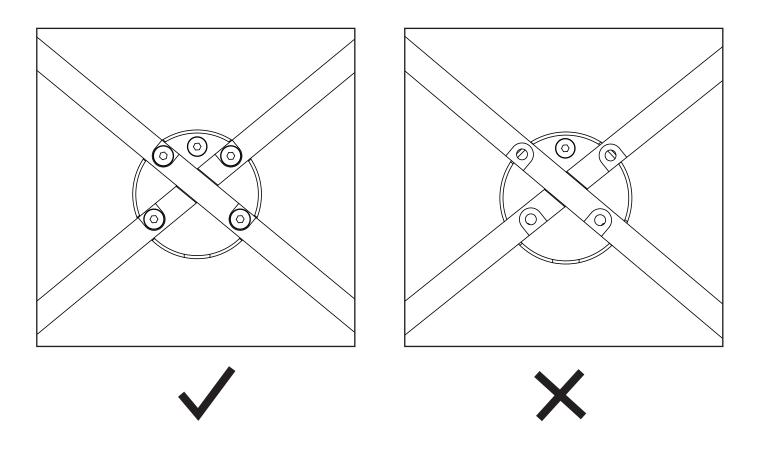
4. Attach the 4 rubber feet onto the legs.
