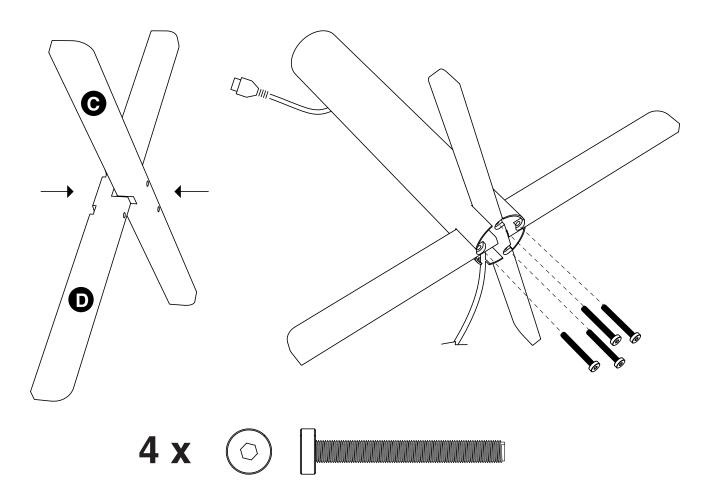
Carefully check that the holes in the legs align with the holes of the steel disc.
