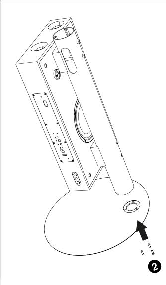
WARNING: Screws must be tight but excess of force can deform the aluminium tube
