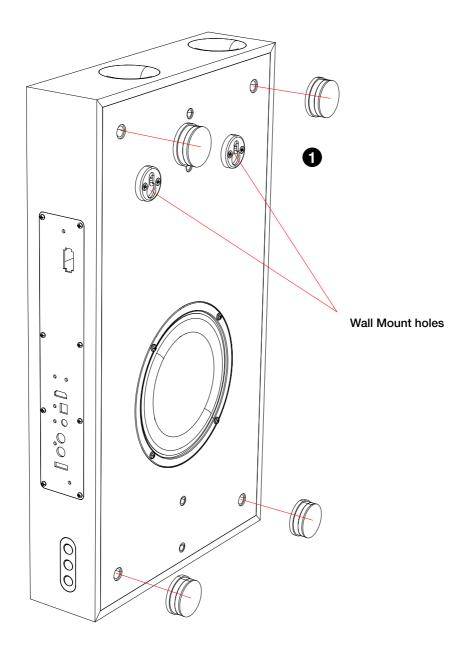
Rubber feet are only needed for a wall mount setup to manage the distance between the Cinema+ and the wall.
